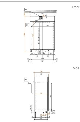
ED = Remote electrical connection RO = Refrigerant Outlet
